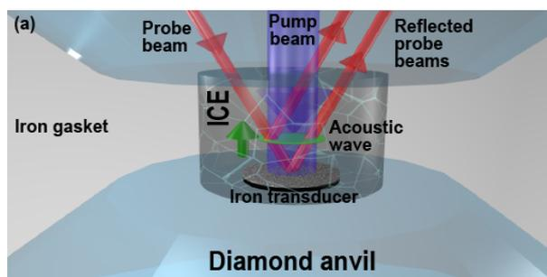
**Fig. Principle of TDBS imaging**
