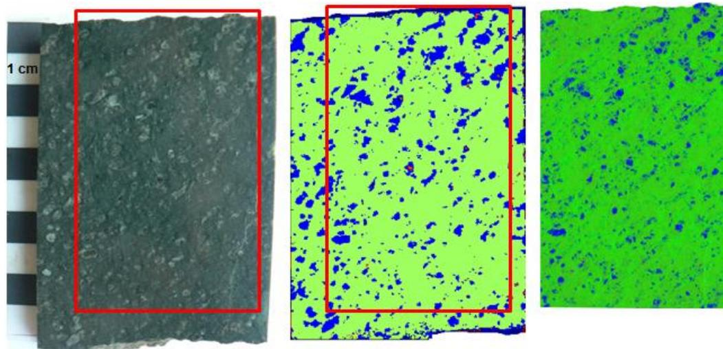
Fig. 4. Results on a serpentinized harzburgite sample. RGB image of the sample (left), unmixing result (middle), QEMSCAN<sup>®</sup> mineralogical mapping (right). Note that the QEMSCAN<sup>®</sup> analysis was done only in the region limited by the rectangle with red border. For the unmixing and QEMSCAN results, the pyroxene, serpentine, chromite and olivine phases are presented in blue, green, red and grey colors, respectively.
