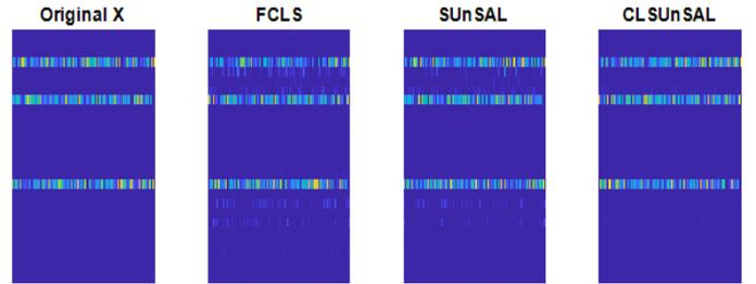
Fig. 3. Generated abundance matrix ( $K = 3$ ) and estimated abundance matrices with three unmixing methods.
