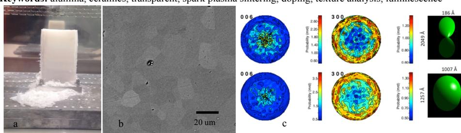
Figure 1. Growing alumina monolith in the climate chamber (a), backscattered electron image of the sintered ceramic (b) and pole figures with crystallite shapes from the XRD texture analysis (c).
