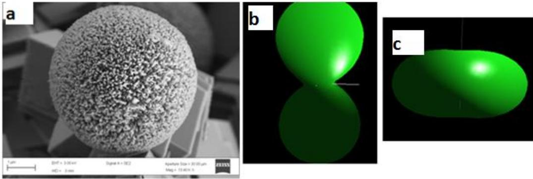
Fig 1: SEM image of vaterite particle (a) vaterite crystallite without PAA (b) vaterite crystallite with PAA.
