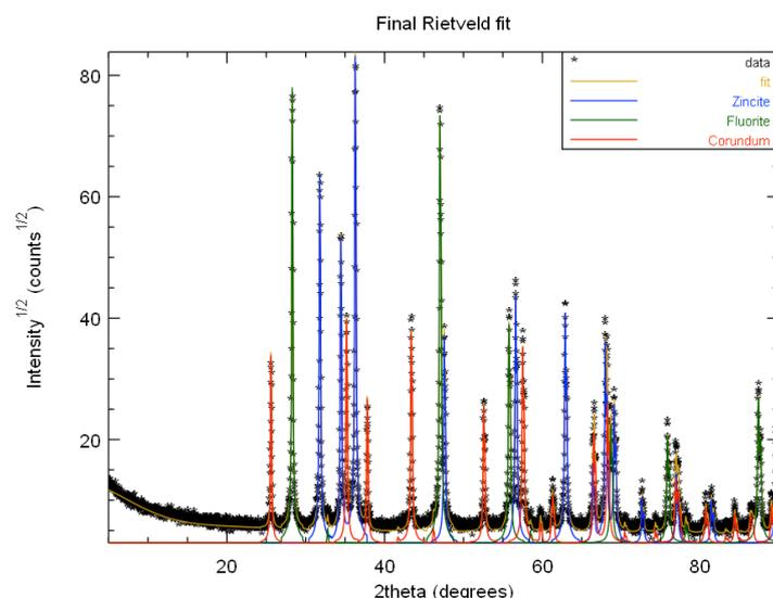
Fig. 1 Table showing the FPSM results for quantitative phase and line broadening analysis on a tri-phase sample, and plot of the fitted pattern with all phases.
