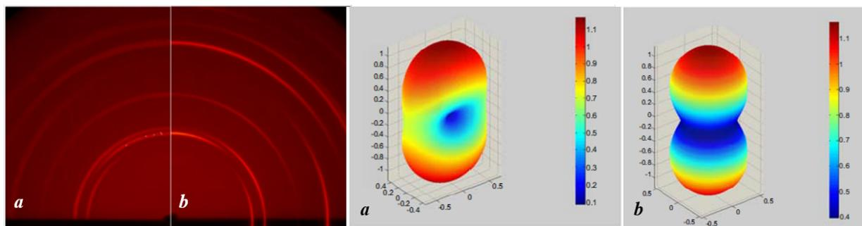
Figure 1: a) Observed and b) calculated 2D-XRD. Figure 2: a) Single- and b) polycrystal magnetoelectric surfaces.
