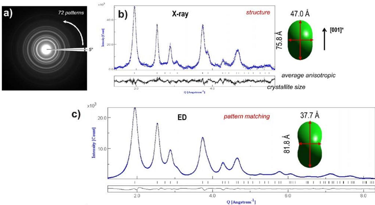
**Figure 1.** a) ED-RP obtained from an assembly of  $\text{TiO}_2$  nanoparticles [3]. The intensity is integrated by sectioning the rings in 72 arcs of  $5^\circ$  extension. b) RX vs. c) ED-RP microstructure analysis (MAUD). The “ED patterns” presented in c) corresponds to the summation of the 72 patterns integrated azimuthally along the rings.
